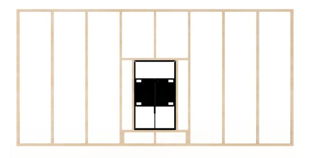
The image above is an example of a bare stud wall with the stand in place. It is vital that you position studs on all four sides of the stand. The stand will screw into each surrounding stud.
