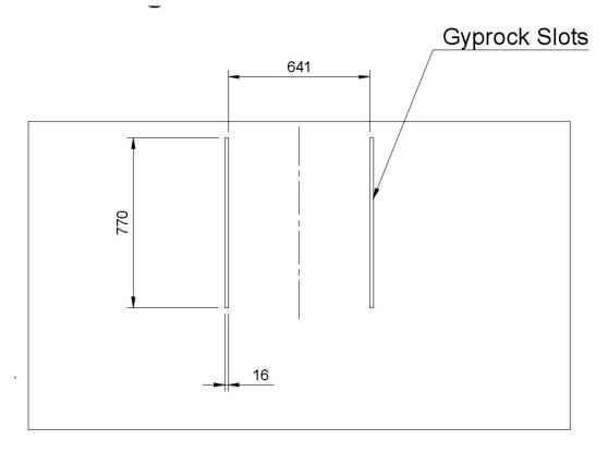
To position the slots, the drawing below shows exactly where the slots should be relative to the corners of the outer frame on the stand. This should help you take accurate measurements.
